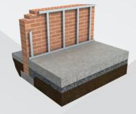
4. Lift the XT/TL-MF into position using wedges on the floor. Insulation should be cut back to accommodate an adjoining panel at external corners. Joints should be tightly butted.
