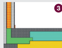
EPS Wrapped Foundation
