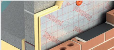
2. Mortar should be struck from the inner cavity face of the block to ensure mortar squeeze is minimised on the cavity side. The two courses of blockwork can then be built, ensuring the mortar is struck back from the cavity face to prevent mortar squeeze.
