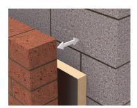
The cavity width is accurate and the cavity insulation has been cut back where the barrier will be located
