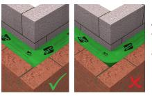
All corners and joints are tightly butt jointed. Barriers are not bent around corners.
