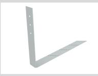
Now bend the spike into an 'L' shape at the fold point (a small 'U' shape cutout on each side).
