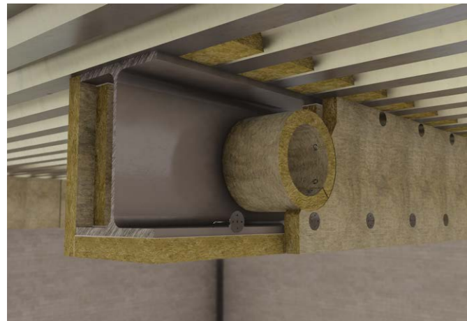
Figure 9 - Beam with circular holes (boxed protection - dry joints)
