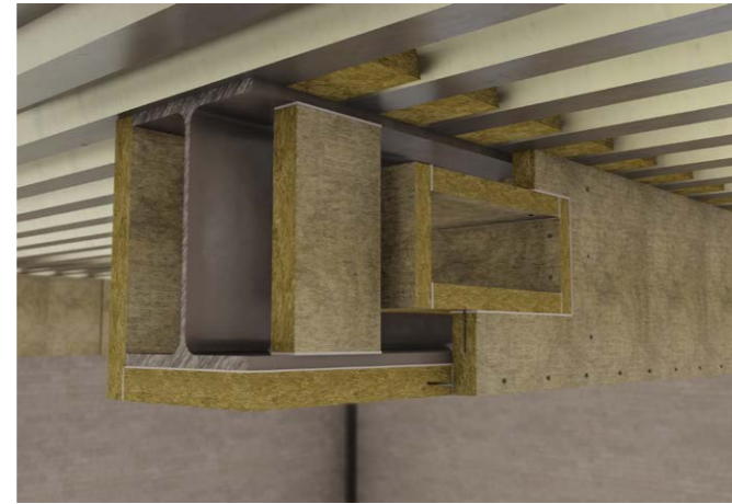
Figure 8 - Beam with square or rectangular holes (boxed protection - glued and pinned joints)
