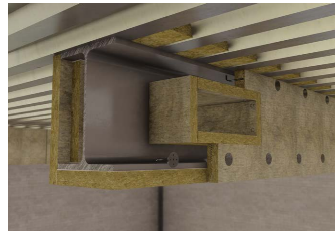
Figure 10 - Beam with square or rectangular holes (boxed protection - dry joints)
