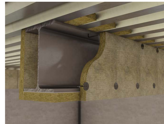
Figure 2 - Stud welded pin dry joint board system (Up to 3 hours fire protection)
