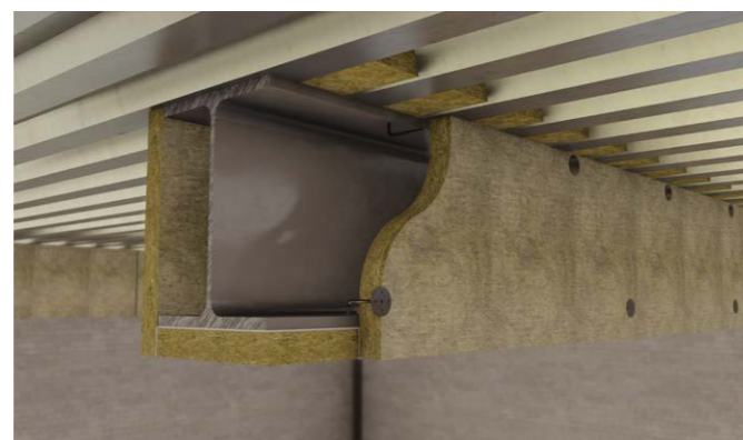
Figure 5 - Stud welded pins and board-to-board glued joints (Up to 4 hours fire protection)
