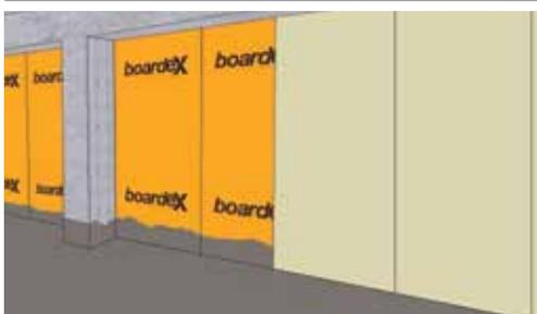
On the inside of exterior walls constructed by **Boardex**, wet applications such as screed and ceramic coating can be carried out before screflange plasterboard. After all these wet productions are finished, **COREX** can be fixed onto the surface of **Boardex** , and the wall surface can be finished.
