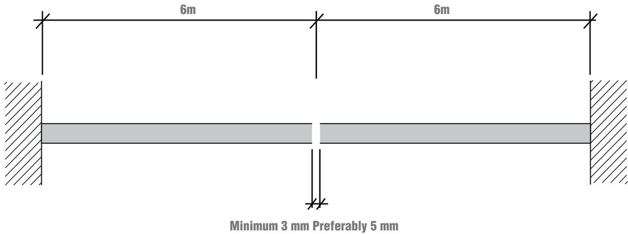
**Figure 3:** Leaving space between box steel profiles
