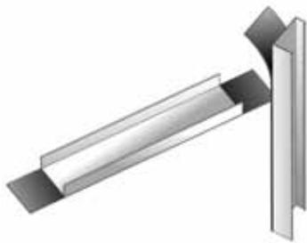
Resilient tape should be affixed underneath the **DU** and **DC** profiles which are fixed on floors, ceilings and walls in order to stop the formation of heat and sound bridges.
