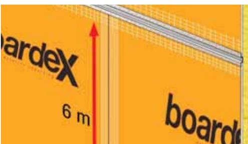
If the **Boardex** surface is coated with mineral plaster, a joint profile with a PVC-based mesh should be used minimum every 6 metres vertically in order to maintain the dilation.
