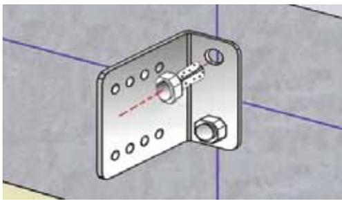
The L brackets should be fixed onto the reinforced concrete flooring by means of steel dowels from two points on a line determined by a guiding string.
