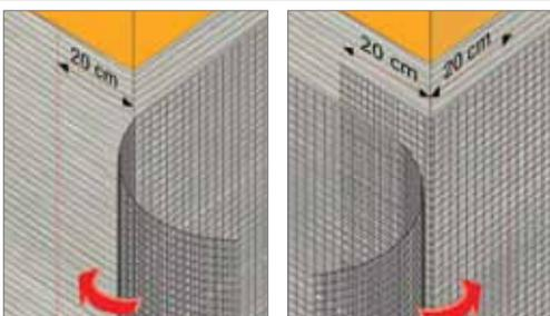
The plaster mesh to be used in the exterior corners should be overlaid 20 cm on both sides.
