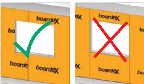
**Boardex** joints in the window cavities should not coincide with the window edge profiles, and the joints should be fixed onto the profiles above or below the lintel.
