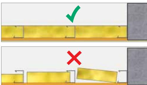
The mineral wools placed between the profiles should be filled in such a way that they do not form any gaps horizontally or vertically.
