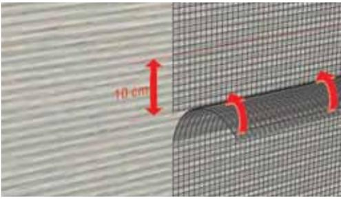
The plaster mesh should overlap around 10 cm at the joints.
