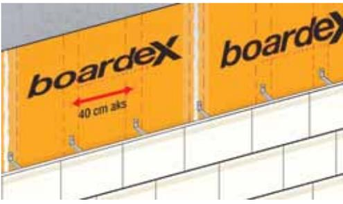
The carrier profiles of the ventilated wall systems are fixed onto the carrier profiles of the **Boardex** exterior wall systems within the range of the axle spacings determined by manufacturing firms, and hence are designed to carry systems weighing 25 kg/m<sup>2</sup>. As far as the ventilated wall systems to be applied onto **Boardex** surfaces are concerned, the advice and application principles of the facade system manufacturers should be taken into account.
