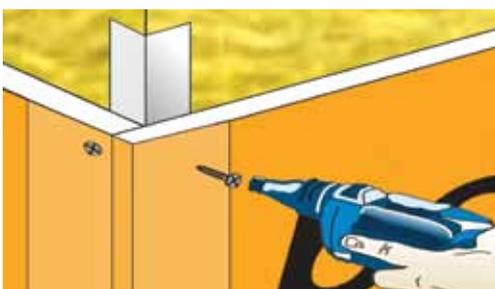
In the corner joints, **Boardex** DKC corner profiles should be applied inside the corner.
