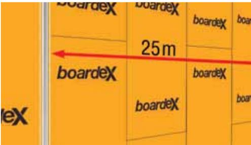
If the **Boardex** surface is coated with mineral plaster, a joint profile with a PVC-based mesh should be used every 25 metres horizontally in order to maintain the dilation.
