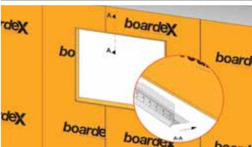
An edging with a PVC-based mesh should be used in the horizontal corners in areas such as eaves, doors and windows.
