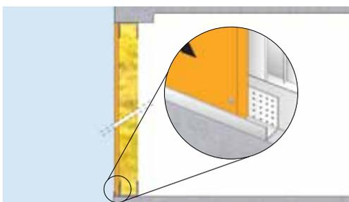
The first **Boardex**, which corresponds to the floor, should be fitted to the PVC-based starter track so that the contact with the floor is cut off.
