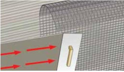
Probaser Render should be applied on all the surface by using a notched trowel. A 160 gr / m<sup>2</sup> alkali-resistant plaster mesh should be placed near the surface to complete the primer before mineral plastering.
