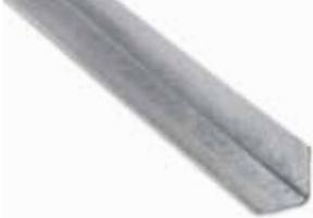
A silver-colored galvanized metal corner profile with an L-shaped cross-section.            | <p>It is a galvanized corner profile, which is 275 gr / m<sup>2</sup> with 0.5 mm thickness that is used to strengthen corners against impact.</p>                                                              |
