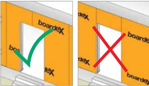
**Boardex** joints in the door cavities should not coincide with the door edge profiles, and the joints should be fixed onto the profiles above or below the lintel.
