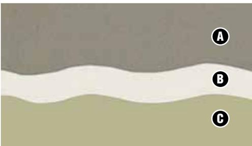
After the prime coat is completed by **Probaser Render** in accordance with the instructions above, for the application of mineral plaster to be applied on this primer coat and for paint application on the mineral plaster, advice and suggestions of mineral plaster and paint manufacturers should be complied with and information about application conditions should be obtained.
