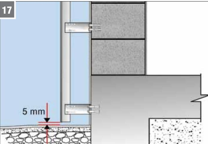
**Connection of BoardeX CT facade profiles on the base**
