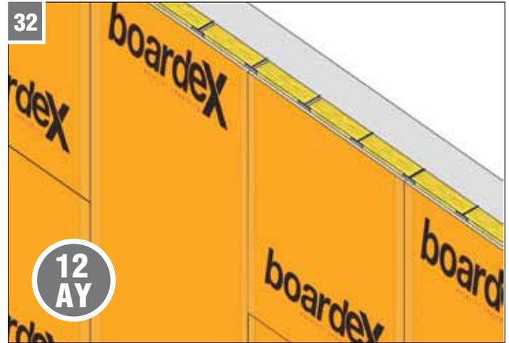
**The surface can be exposed to the atmosphere for up to 12 months**
