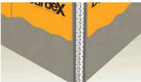
If the **Boardex** surface is coated with mineral plaster, a corner profile with a PVC-based mesh should be used for the exterior corner joints.
