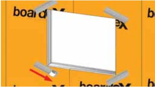
In order to reduce the risk of cracking in the corners of the window cavities, a joint tape should be applied in a cross manner and be covered by **Probase Render**.
