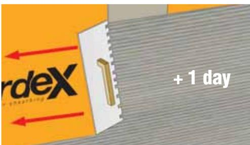
The primer coat application should be carried out at least 1 day after the joint application is completed.
