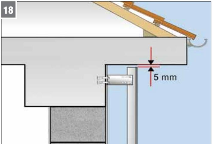
**Connection of BoardeX CT facade profiles on the ceiling**
