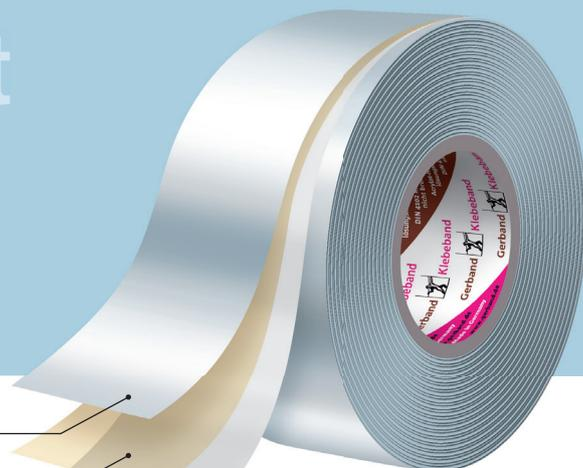
Gerband 712 is an aluminum film tape with a strong adherent, strongly cross-linked polyacrylate adhesive with high ageing resistance and good shear strength. It is used for applications under high temperature load as well as for masking, insulation and sealing.
