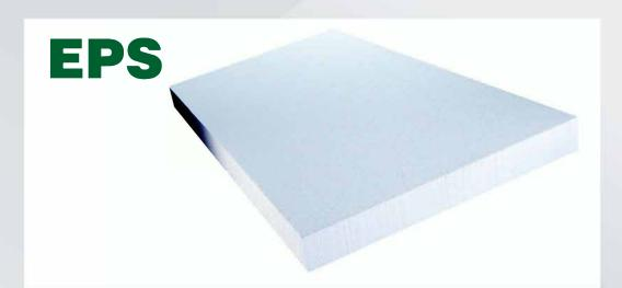
The Xtratherm Warm-R & Warm-R Premium Insulation Boards consists of rigid polystyrene boards cut from moulded blocks of white EPS (Warm-R) or with grey graphite enhancement (Warm-R Premium). The boards are manufactured in square edge, T&G and shiplap jointing. Xtratherm Warm-R & Warm-R Premium Insulation Boards are installed during construction.
