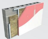
3. Fix the metal frame system/vertical timber battens at a maximum of 600mm centres (incorporating a vertical DPC behind timber battens). Ensure framing system/battens are wide enough to offer 20mm support to all four edges of the plasterboard. Pack battens if necessary to level the wall. Extra noggins may be required when the Safe-R Fireline Thermal Laminate is unsupported by the battens.
