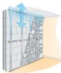
Fig 4: Height adjustable metal studs
